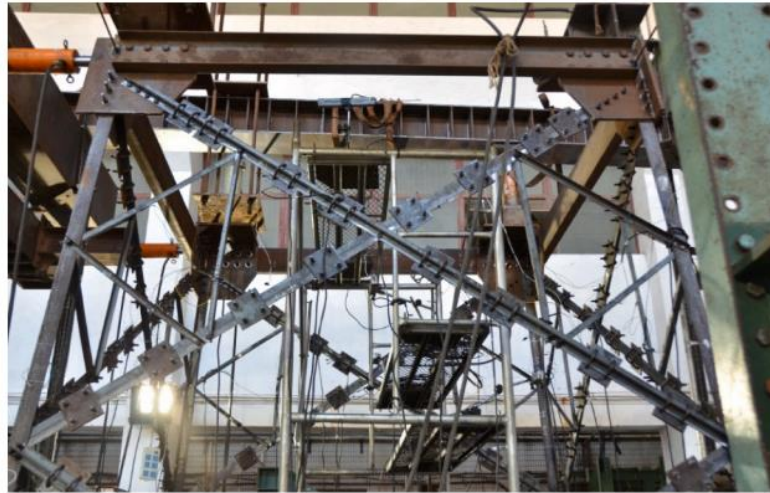
Fig. 2. Retrofitting system and the retrofitted sub-assembly. [11].
