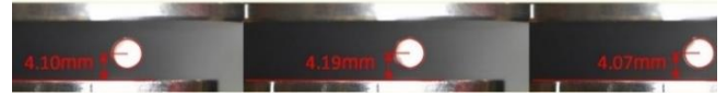
Fig. 5. Movement analysis of the levitated particle in three successive frames of the video recording in the experiments.
