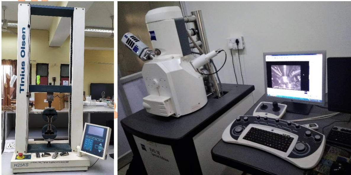
Fig. 6. UTM was used for tensile and flexural tests, and SEM was used for fracture behavior characterization.
