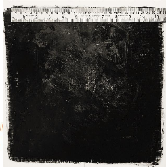
Fig. 4. A composite plate fabricated through a vacuum pump assists the hand lay-up method.
