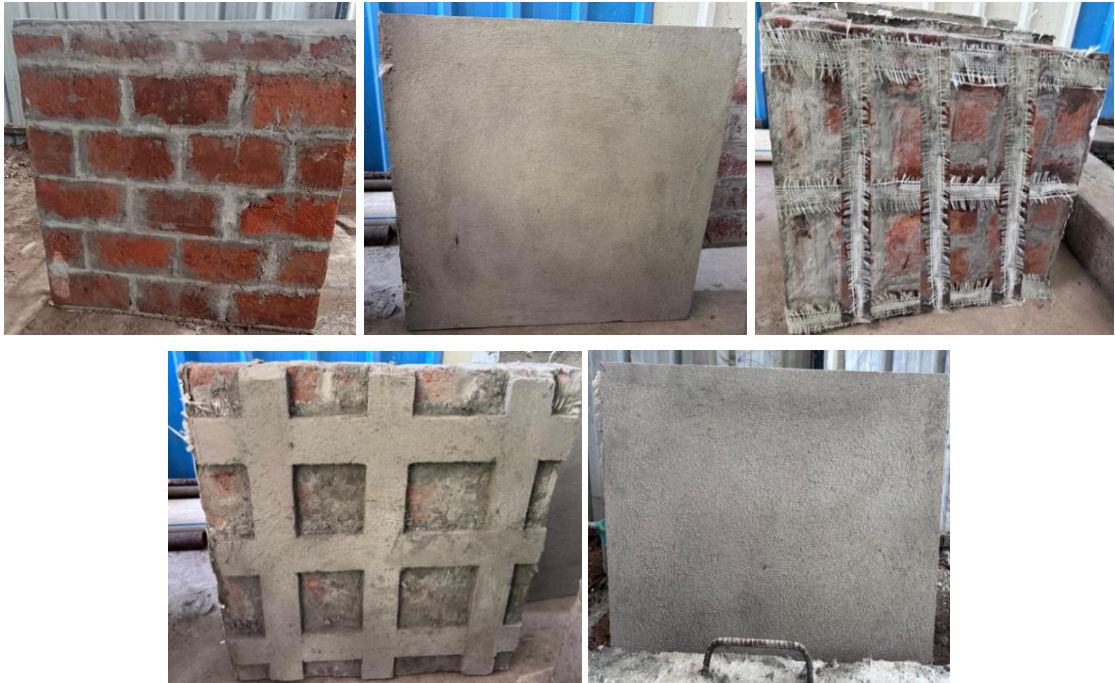
(b) Brick Masonry wallets after strengthened.
