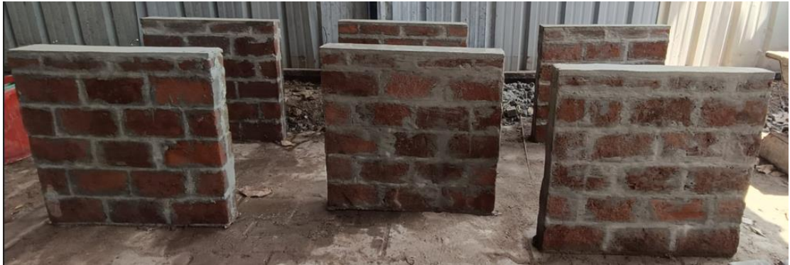
(a) Brick Masonry wallets before strengthening.
