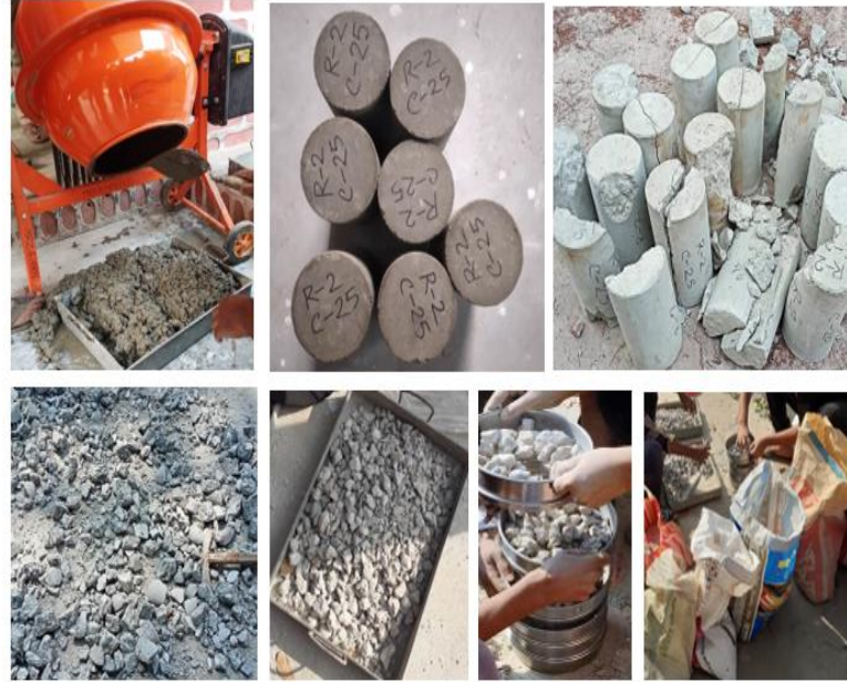
Fig. 4. Concrete specimen preparation and testing.
