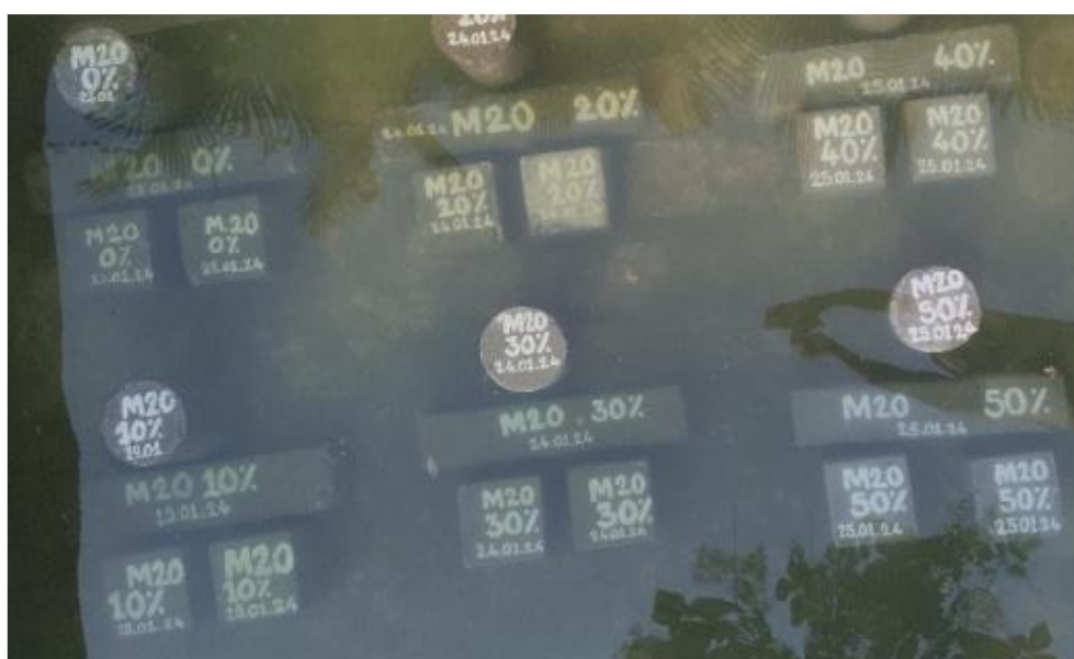
Casted Specimen samples
