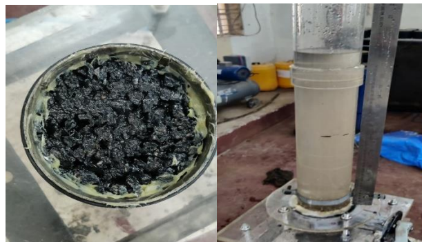
Fig. 7. a) porous asphalt sample ready for test; b) 24-hour saturation before conducting a test (permeameter filled with water).
