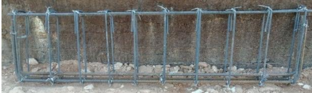
Fig. 1. Detailing of steel reinforcement of the tested specimens.
