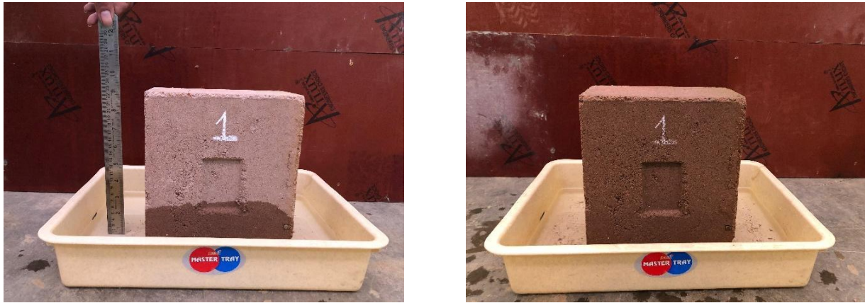
Fig. 16. Test setup for the blocks placed for efflorescence.
