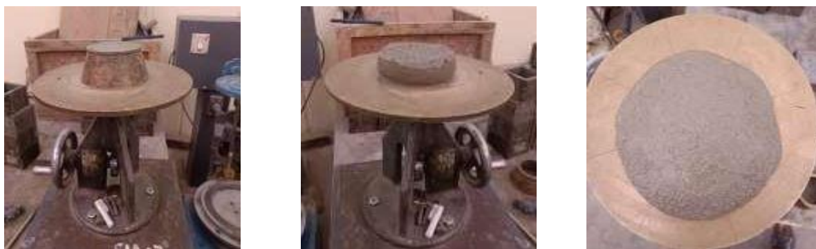
Fig. 18. Flow table test and nature of flow of mortar.
