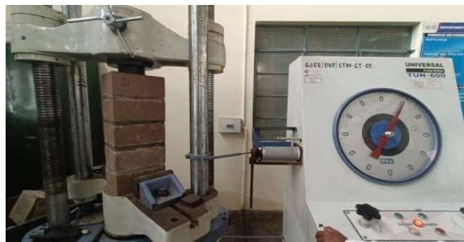
(b): Testing of Specimen in compression testing machine.
