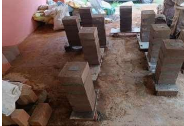
(a): Masonry prisms made of masonry blocks in the casting yard.
