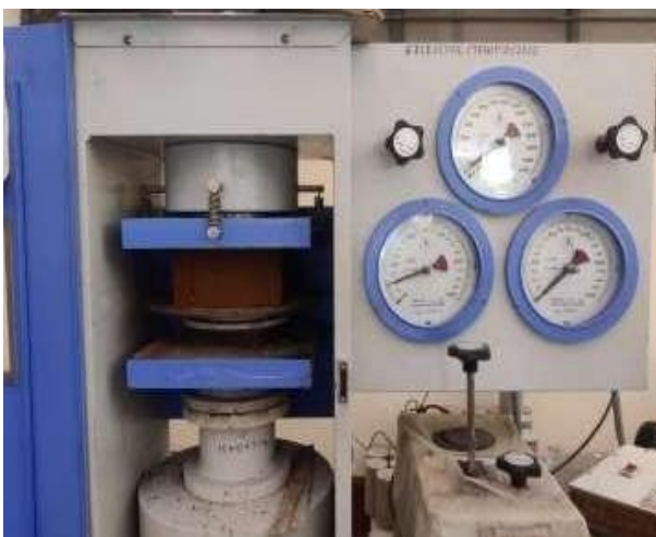
(a) Block placed in compression testing machine.
