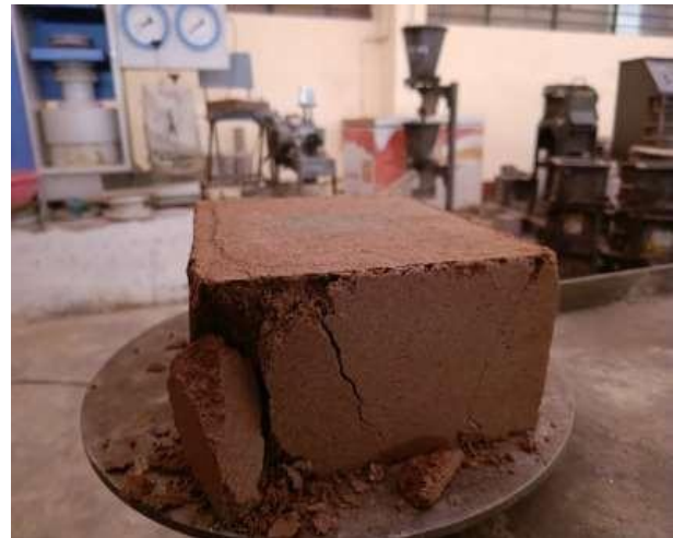
(b) Failure pattern of the tested specimen.
