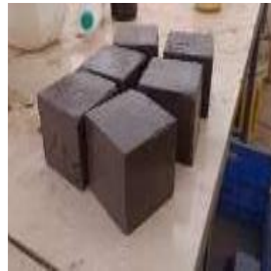
(b) Demoulded cubes of size 70.7 mm.
