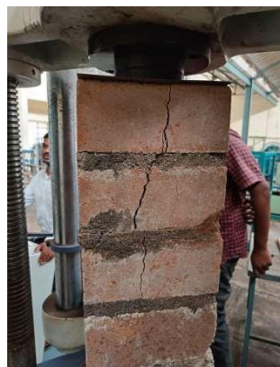
(c): Nature of failure.
