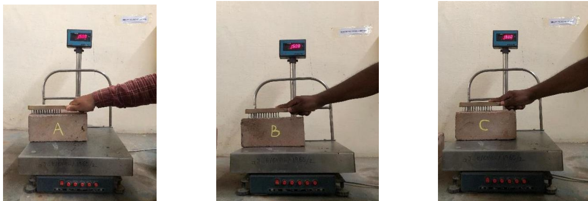
Fig. 23. Samples considered for the weathering test and measure of applied pressure by wire brush scratch.
