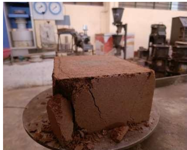
(b) Failure pattern of the tested specimen.
