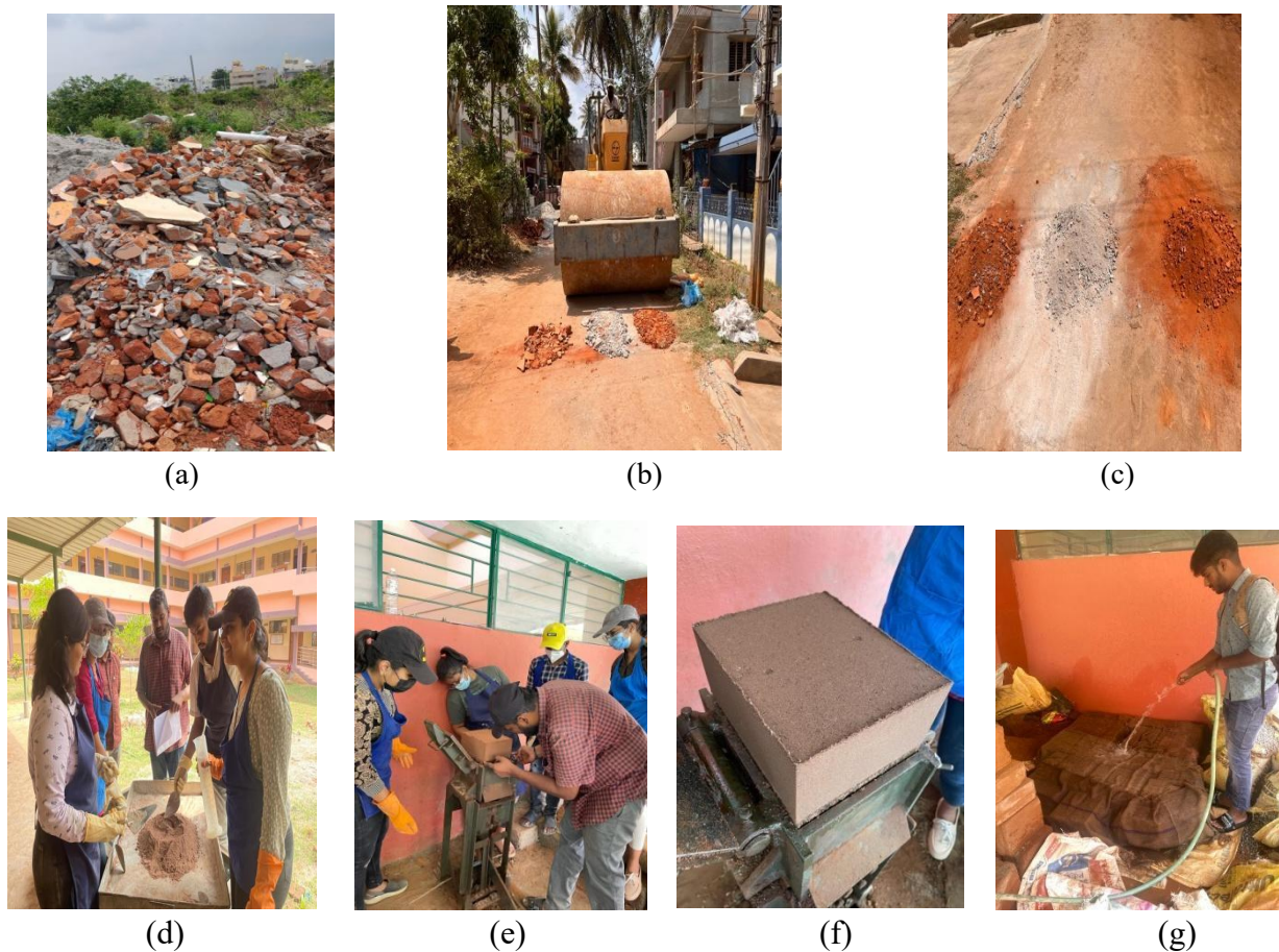
Fig. 4. shows the manufacturing process of the Recycled Aggregate (RA) blocks. (a) Demolished Masonry is used in landfills. (b) Grinding of waste by road roller (c) Ground powder of CDW collected from nearby landfills. (d) Sieving and proportioning of RA. (e) and (f) Manufacturing of RA blocks using a manual compression machine. (g) Samples are cured by water spraying at regular intervals on the blocks.
