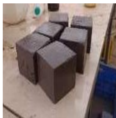
(b) Demoulded cubes of size 70.7 mm.
