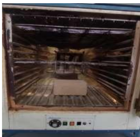
(a): Oven drying of block.
