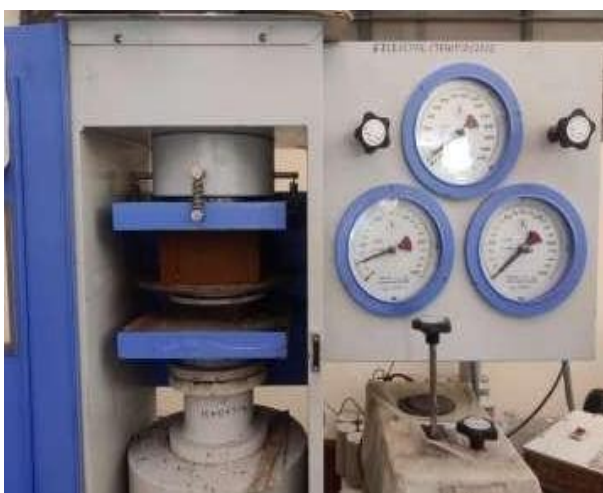
(a) Block placed in compression testing machine.
