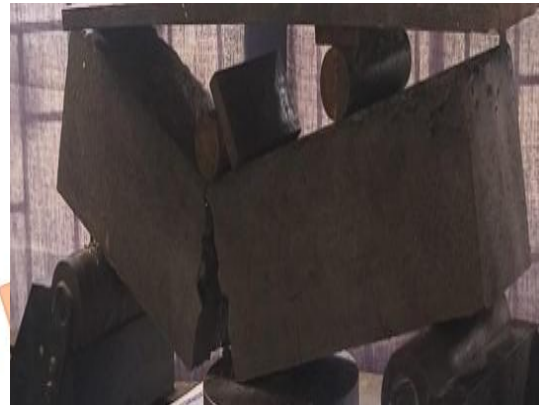
Fig. 16. Specimen (Solar dried with PCM) after Flexural Strength test
