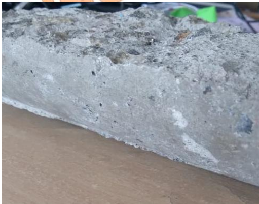
Fig. 14. Specimen (Solar dried with PCM) after Tensile test
