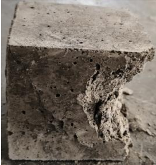
Fig. 14. Specimen (Solar dried with PCM) after Tensile test
