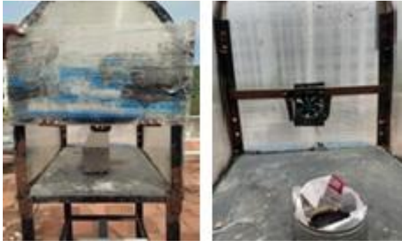
Fig. 6. Novel GPB along with (PCM) Ferric Chloride Dihydrate in a solar dryer
