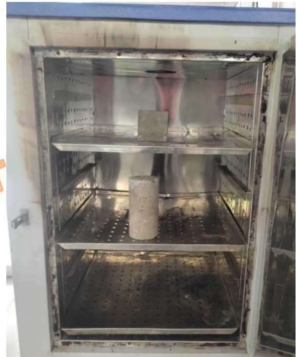
Fig. 5. Novel GPB (cubic and cylindrical) specimen kept in an electric oven.
