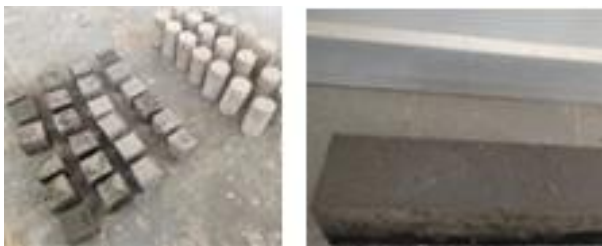
Fig. 4. (a) Specimen for tensile (cubic) & compressive (cylindrical) testing, (b) Specimen for flexural testing
