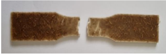
Fig. 4. PP/DPF sample after tensile test
