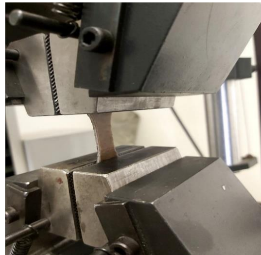
Fig. 3. Tensile sample of PP/DPF composite undergoing tensile test inside the clamps of the machine
