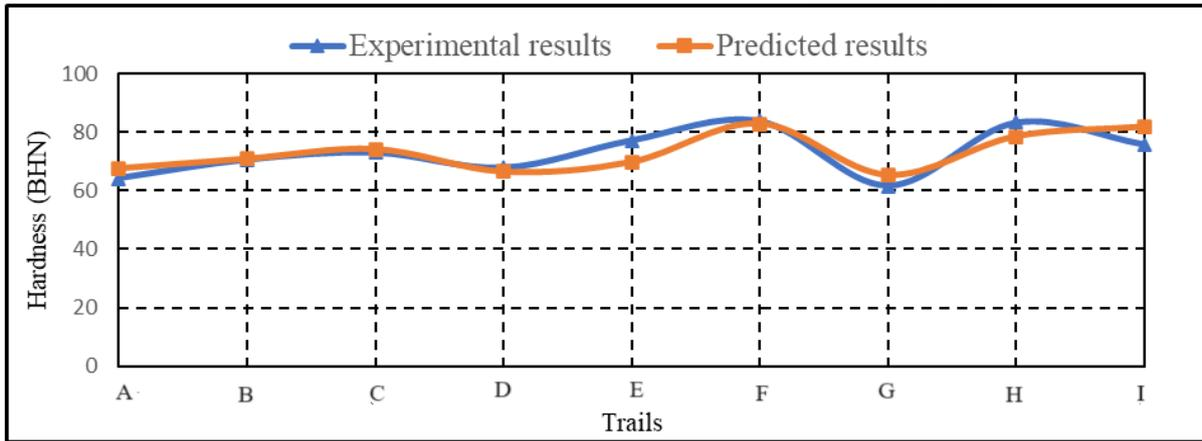
Fig. 13. (a) Graph of experimental hardness and predicted results of hardness for AW2024/B<sub>4</sub>C composite.
