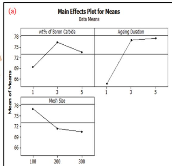
Fig. 12. (a) Optimization of the BH number of AW2024/B<sub>4</sub>C reinforced composite.
