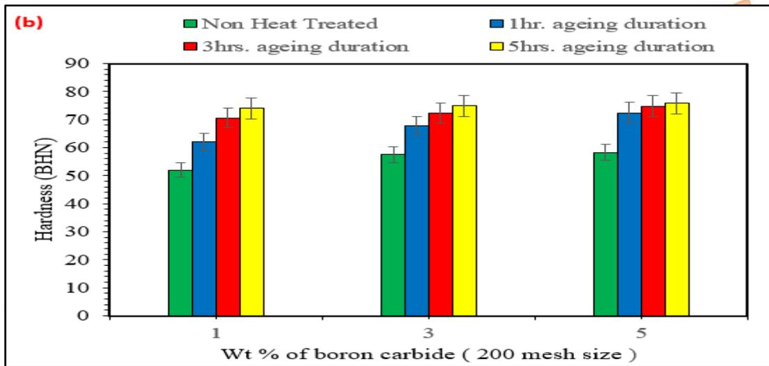
Fig. 10. (b) Plot of Hardness for different AW2024/B<sub>4</sub>C composites (200 mesh size of B<sub>4</sub>C)
