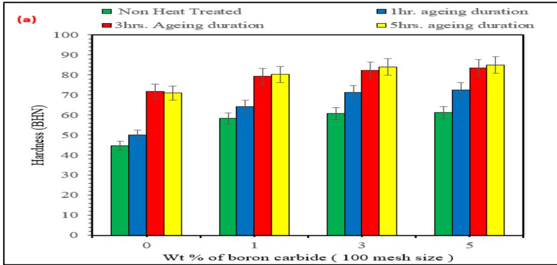
Fig. 10. (a) Plot of Hardness for different AW2024/B<sub>4</sub>C composites (100 mesh size of B<sub>4</sub>C)
