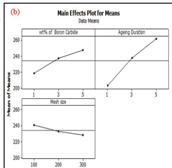
**Fig. 12. (b)** Optimization of Tensile strength of AW2024/B<sub>4</sub>C reinforced composite.
