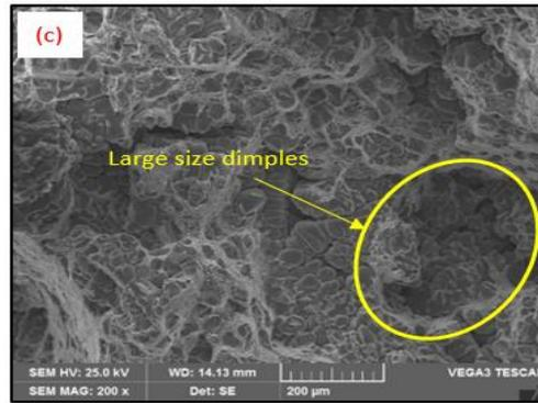
**Fig. 14.** Tensile fracture SEM images for (a) AW2024/3 wt.% B<sub>4</sub>C reinforced composite (100 mesh-size) (b) AW2024/3 wt.% B<sub>4</sub>C reinforced composite (200 mesh-size) (c) AW2024/3 wt.% B<sub>4</sub>C reinforced composite (300 mesh-size)
