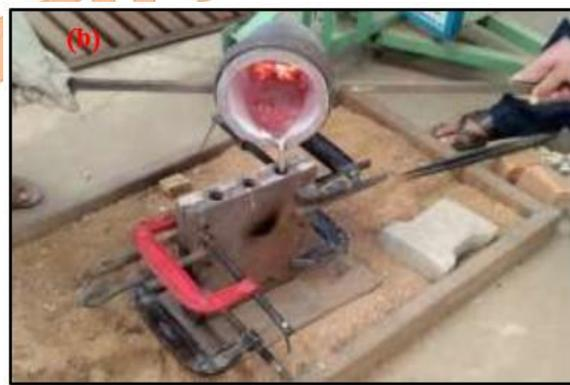
**Fig. 3.** Experimental setup for HMMC's: (a) Electric furnace.
