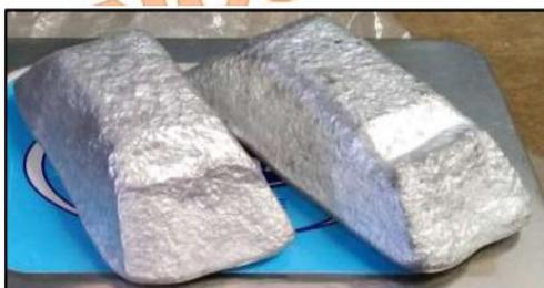
Figure 1. Ingots of AW2024 matrix alloy.
