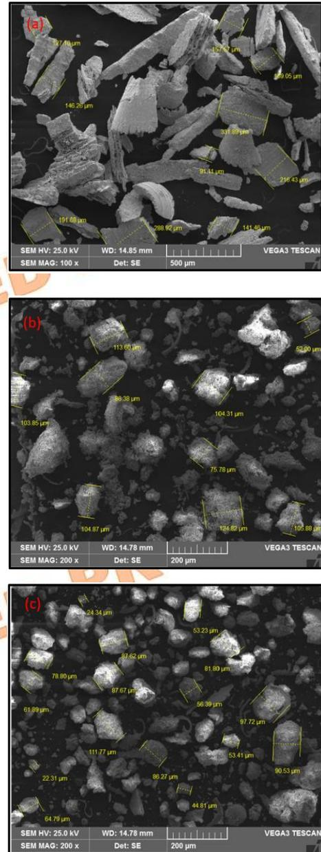
Fig. 2. SEM photograph of B<sub>4</sub>C particles. (a) 100 mesh-size (b) 200 mesh-size (c) 300 mesh-size.
