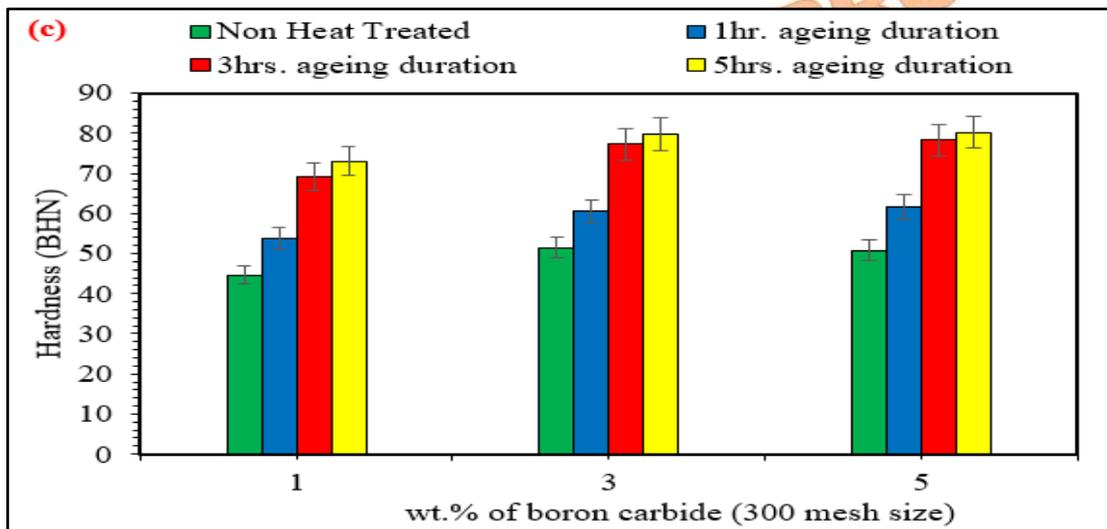
Fig. 10. (c) Plot of Hardness for different AW2024/B<sub>4</sub>C composites (300 mesh size of B<sub>4</sub>C)
