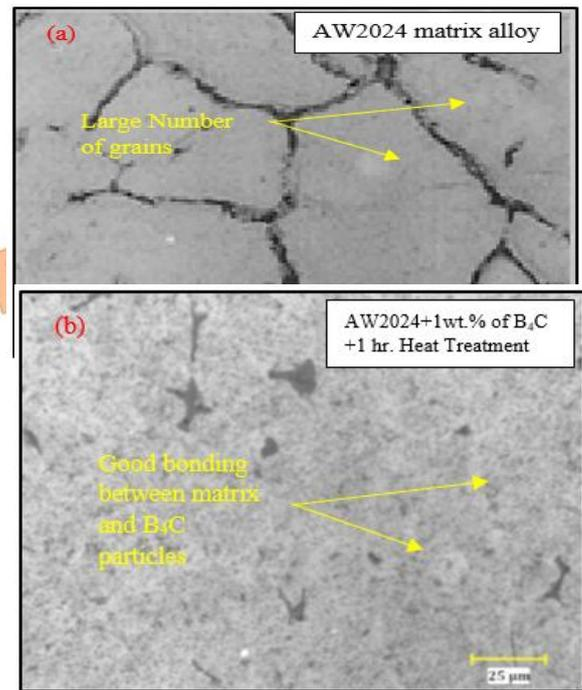
**Fig. 9. (a-d)** Microstructure photograph of AW2024/ $B_4C$  composite for different heat treatment durations.
