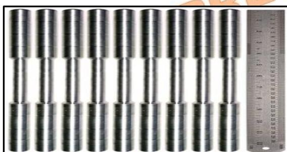
Fig. 4. AW-2024/B<sub>4</sub>C composite -Tensile test samples
