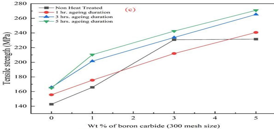
Fig. 11. (c) Tensile strength plot for different AW2024/B<sub>4</sub>C composites (300 mesh-size of B<sub>4</sub>C)
