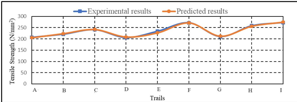
Fig. 13. (b). Graph of experimental and predicted results of tensile strength for AW2024/B<sub>4</sub>C composite.
