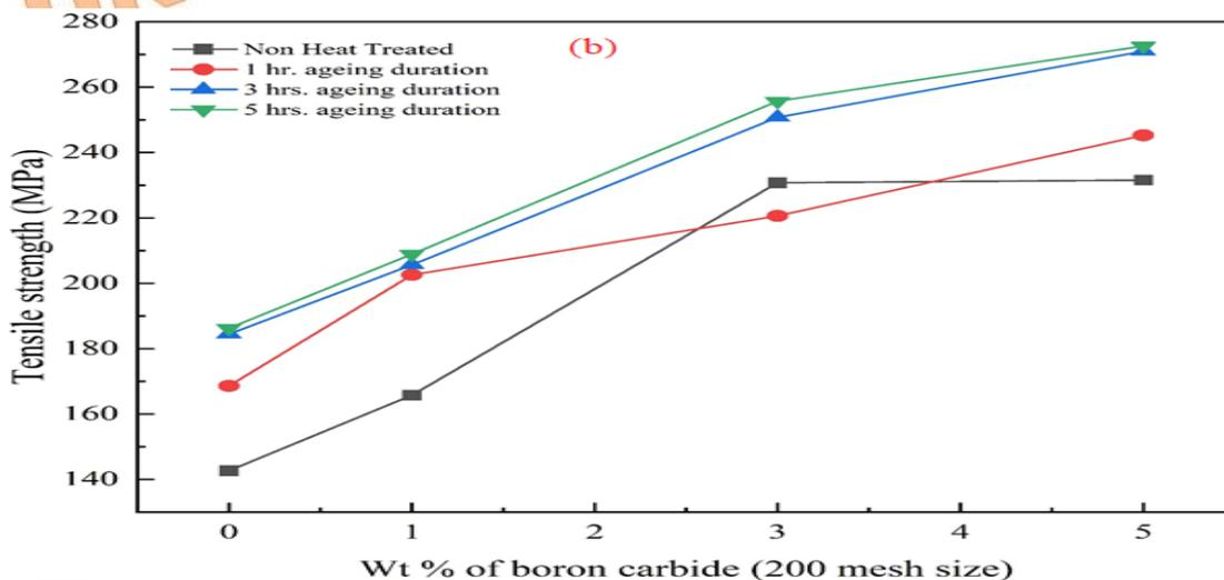
Fig. 11. (b) Tensile strength plot for different AW2024/B<sub>4</sub>C composites (200 mesh-size of B<sub>4</sub>C)
