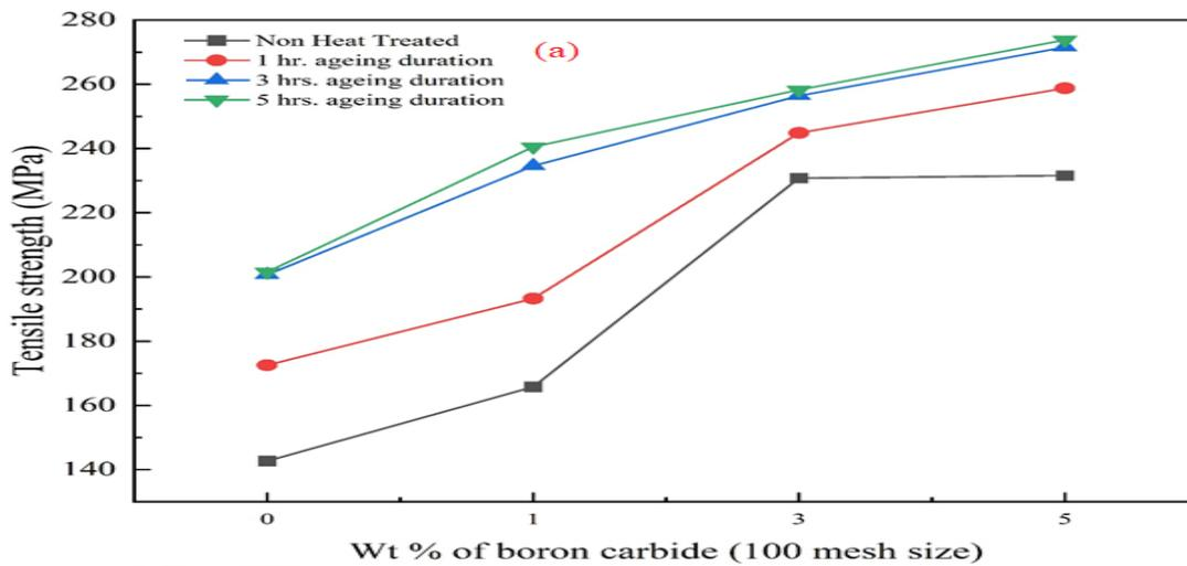
Fig. 11. (a) Tensile strength plot for different AW2024/B<sub>4</sub>C composites (100 mesh-size of B<sub>4</sub>C)
