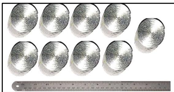
Fig. 5. AW-2024/B<sub>4</sub>C composite - Hardness test samples.
