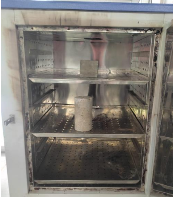
Fig. 5. Novel GPB (cubic and cylindrical) specimen kept in an electric oven
