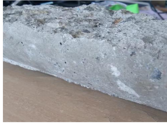
Fig. 15. Specimen (Solar dried with PCM) after Compression Strength test
