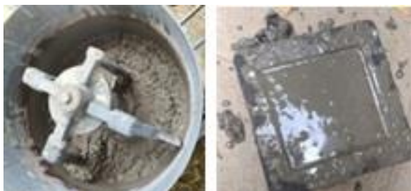
Fig. 3. (a) Final mixture, (b) mixture poured into mold
