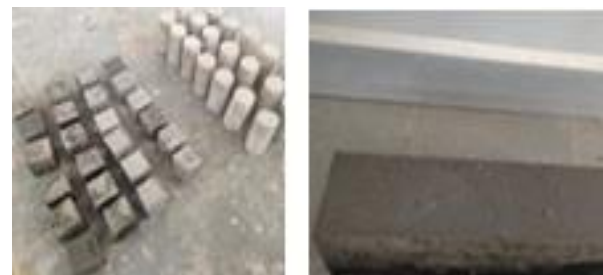
Fig. 4. (a) Specimen for tensile (cubic) & compressive (cylindrical) testing, (b) Specimen for flexural testing
