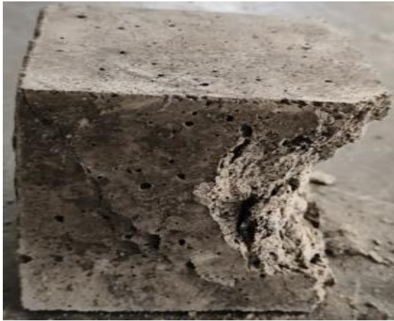
Fig. 14. Specimen (Solar dried with PCM) after Tensile test
