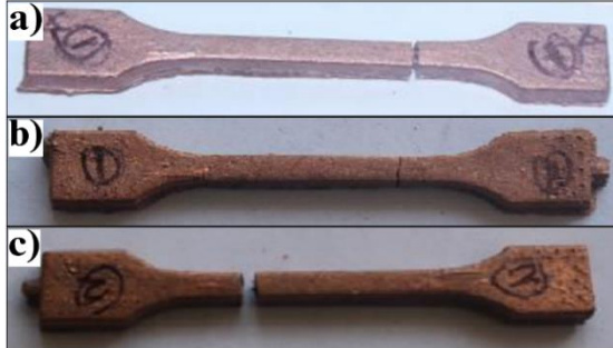
Fig. 5. (a) ABS-Cu (65% ABS + 60% Copper) after the tensile test, (b) ABS-Cu (44% ABS + 50% Copper) after the tensile test, and (c) ABS-Cu (23% ABS + 70% Copper) after the tensile test
