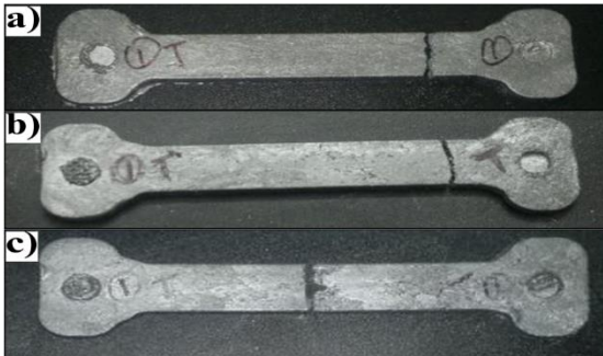
Fig. 6. (a) ABS-Al (65% ABS + 30% aluminium) after the tensile test, (b) ABS-Al (44% ABS + 50% aluminium) after the tensile test, and (c) ABS-Al (23% ABS + 70% aluminium) after the tensile test
