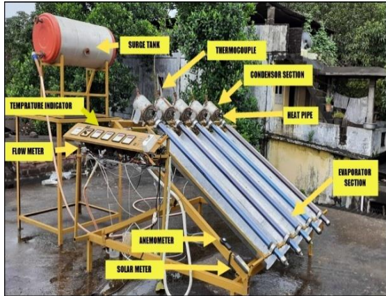
Fig. 2. Experimental setup of HPETSC
