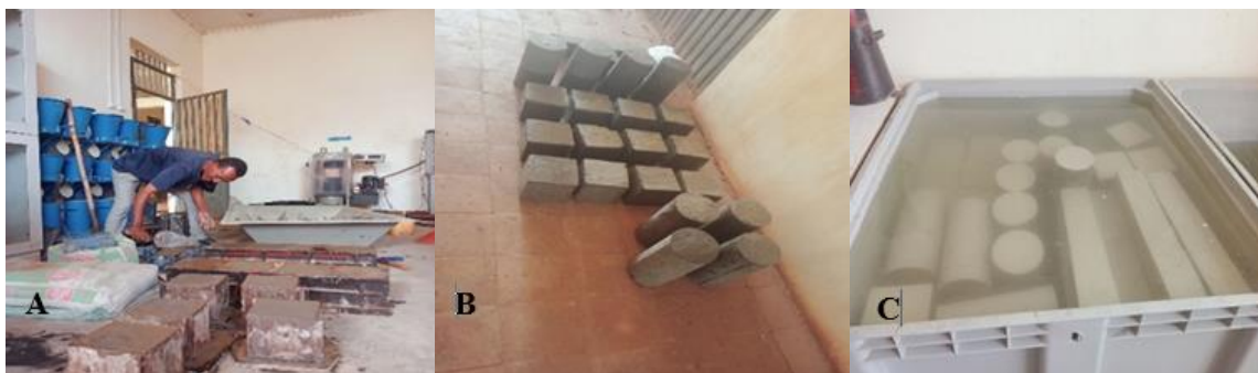
Fig.3. Preparation of specimens and curing.
