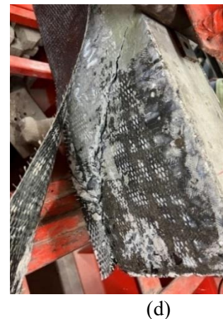
Fig. 9. Behaviour of Beams Second Set of Beams (a) Load vs Deflection (b) Cracks in Normal beam without FRP wrapping (c) Experiment of beam with wrapping (d) Failure of beam after wrapping.
