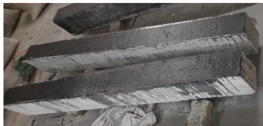
Fig. 3. Two layers of FRP at the bottom surface of the beam.
