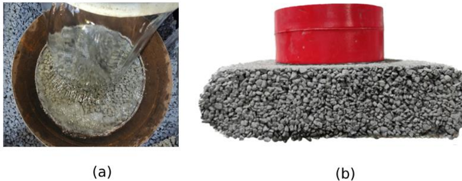
Fig. 4. Permeability test setup using a steel infiltration ring placed on the surface of a pervious concrete slab.
