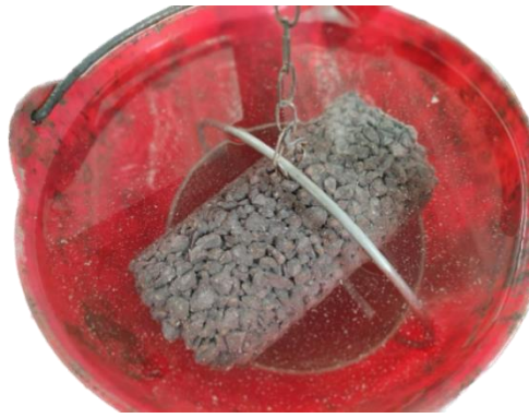
Fig. 6. Porosity measurement using buoyancy method and submerged weight apparatus.
