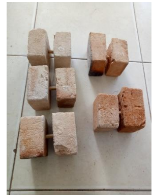
Installing rattan on the compression test object
