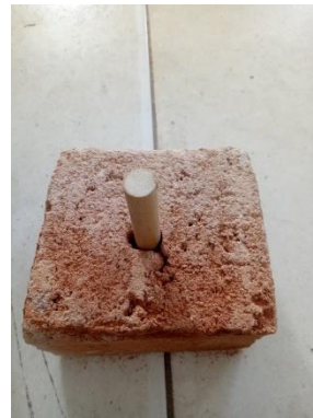
Installing rattan on brick
