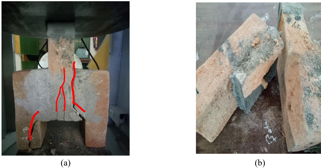
Fig. 14. Damage pattern of shear test specimens; (a) Crack pattern, and (b) Rattan separated from the brick.
