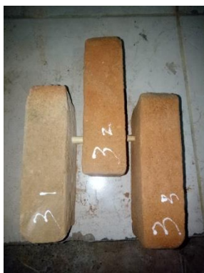
Installing rattan on the shear test object
