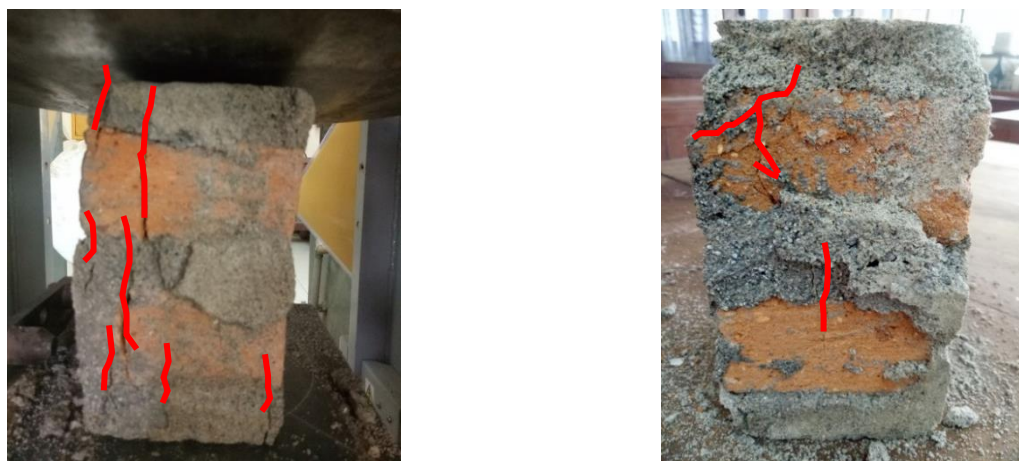
Fig. 12. Crack pattern of compression test specimens.
