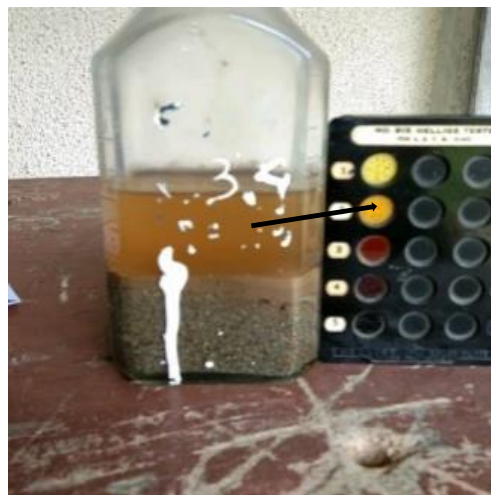
Fig. 9. Sand organic substance test results.
