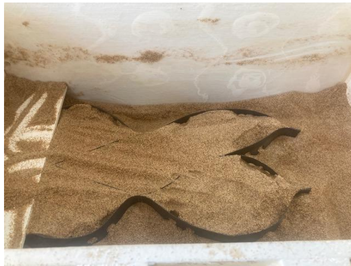
Fig. 4. Geocell placement in pullout box.
