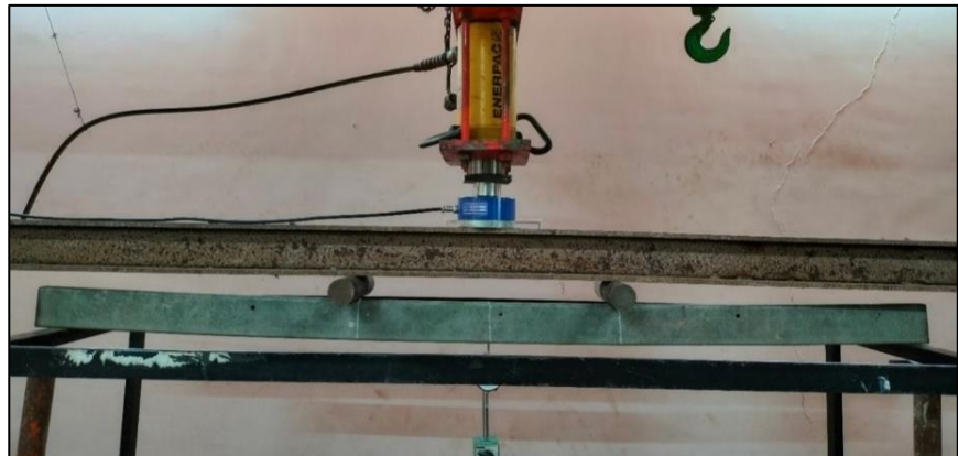
Fig. 3. Experimental Setup: (a) Tensile Testing of Plates, (b) Flexural Testing of Channel Section.
