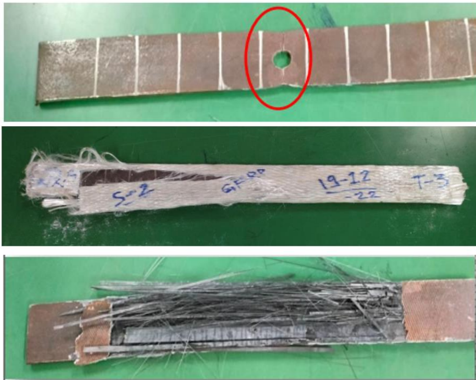
Fig. 7. Failure Modes for Grooved Steel Plates: (a) NP-G local yielding and tearing at hole edge, (b) GFRP-DL-Grooved gradual fiber rupture and adhesive shear-out, and (c) CFRP-DL-Grooved localized laminate cracking and partial delamination near groove location.
