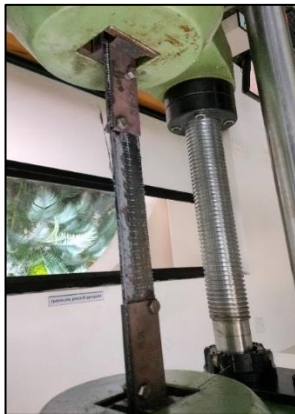
Fig. 3. Experimental Setup: (a) Tensile Testing of Plates, (b) Flexural Testing of Channel Section.
