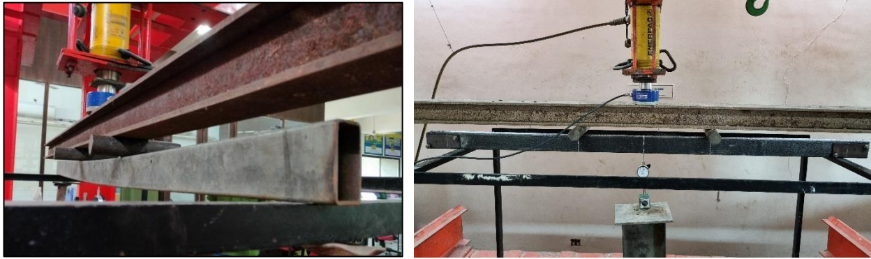
Fig. 9. Flexural Testing (a) Beam without FRP, (b) Beam with FRP.
