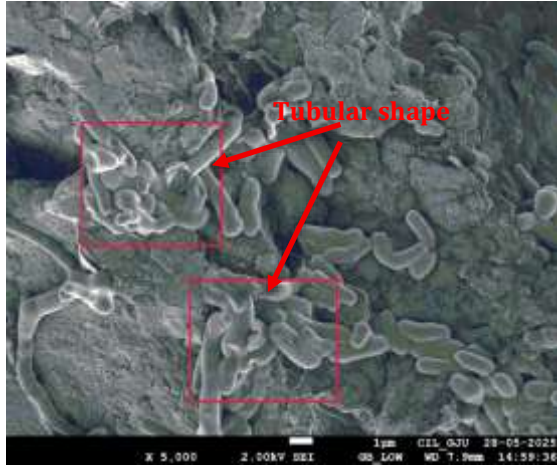
Fig. 4 (a). SEM images of the soil sample treated with MSWIA and nano zeolite
