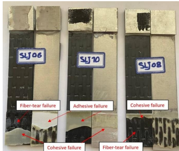
Fig. 12. Mix failure pattern in specimens after the tensile test
