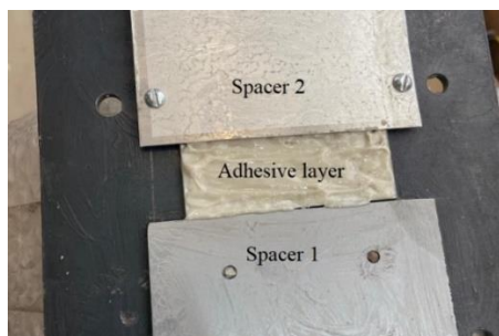
Fig. 2. (b) Produced fixture
