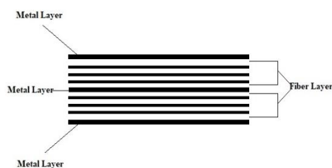
Fig. 1. Schematic sketch of Fiber Metal Laminate showing Fiber and Metal layers for the 3/2 configuration
