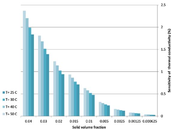
Fig. 8. Sensitivity analysis of thermal conductivity predicted by the experimental model “3” at different temperatures and concentrations
