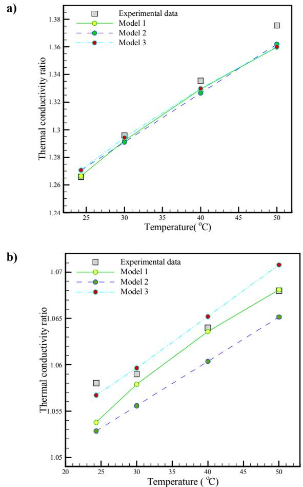
Fig. 4. comparison between experimental data and proposed correlations at a) φ = 5% , b) φ = 1%
