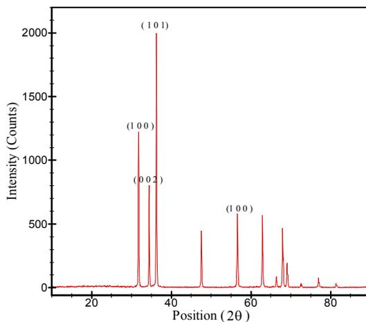
Fig. 1. TEM image and XRD patterns of ZnO nanoparticles
