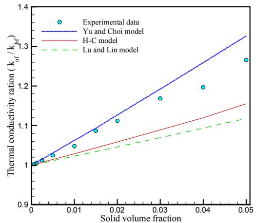
Fig. 2. Comparison between theoretical models and experimental data
