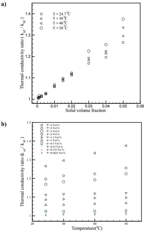
Fig. 3. Thermal conductivity ratio a) at different temperature versus solid volume fraction b) for various concentration with respect to temperature
