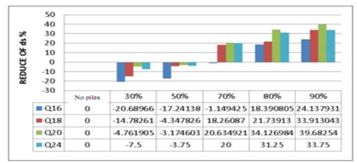
**Fig. 8.** The diagram of reduce of volume and the maximum scour depth according to the submergence percentages of piles
