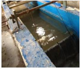
Fig. 2. The valve used to adjust the tailwater depth
