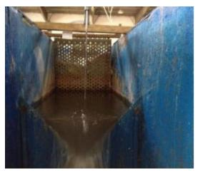
Fig. 1. Triangular weir for flow measurement
