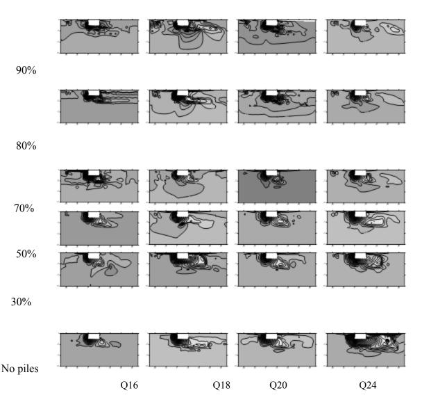
Fig. 6. Bed profile at different flow rates and different submergence percentages
