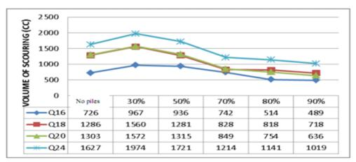
Fig. 7. The diagram of the maximum volume of scour and depth of scour according to the submergence percentages of piles
