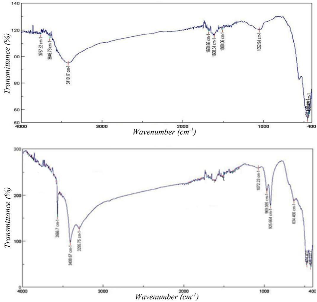
Fig. 2 FTIR spectra of (a) undoped and (b) Fe doped SnO<sub>2</sub> samples
