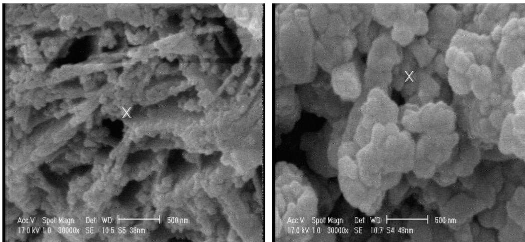
Fig. 3 SEM images of (a) undoped and (b) Fe-doped (7.93 wt%) SnO<sub>2</sub>
