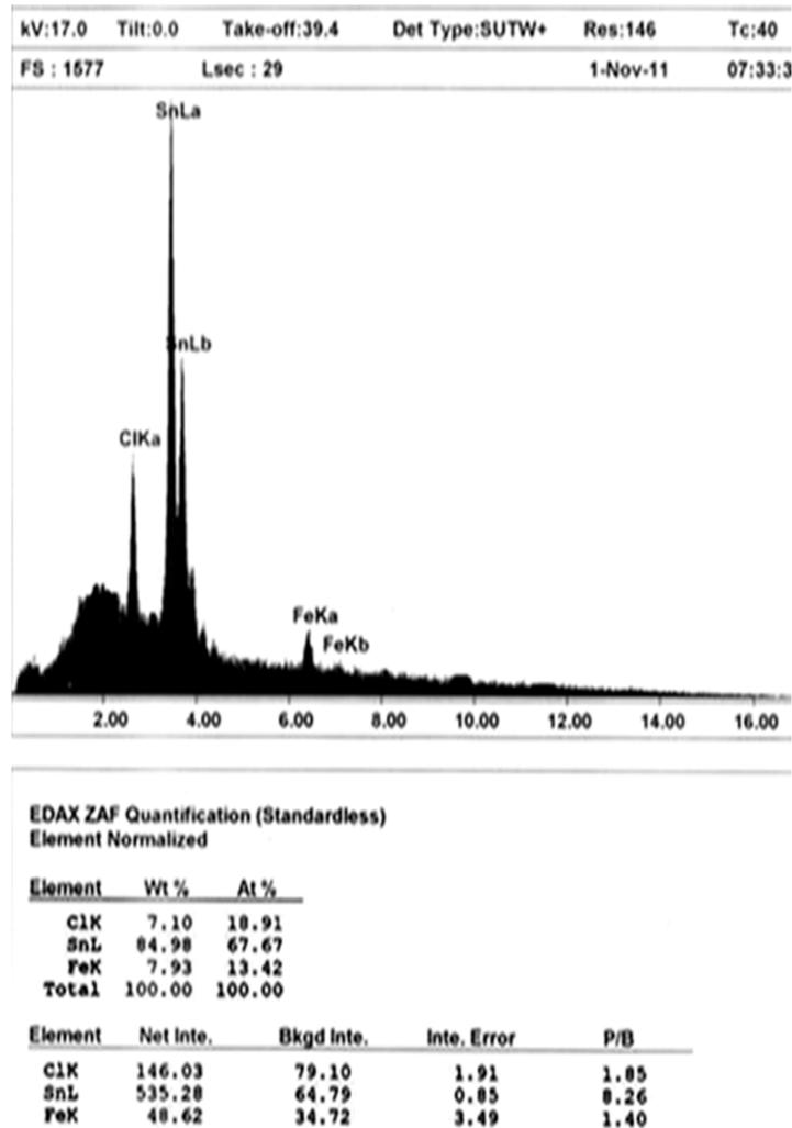
Fig. 4 EDX pattern for Fe-doped SnO<sub>2</sub> (7.93 wt %) nanoparticles
