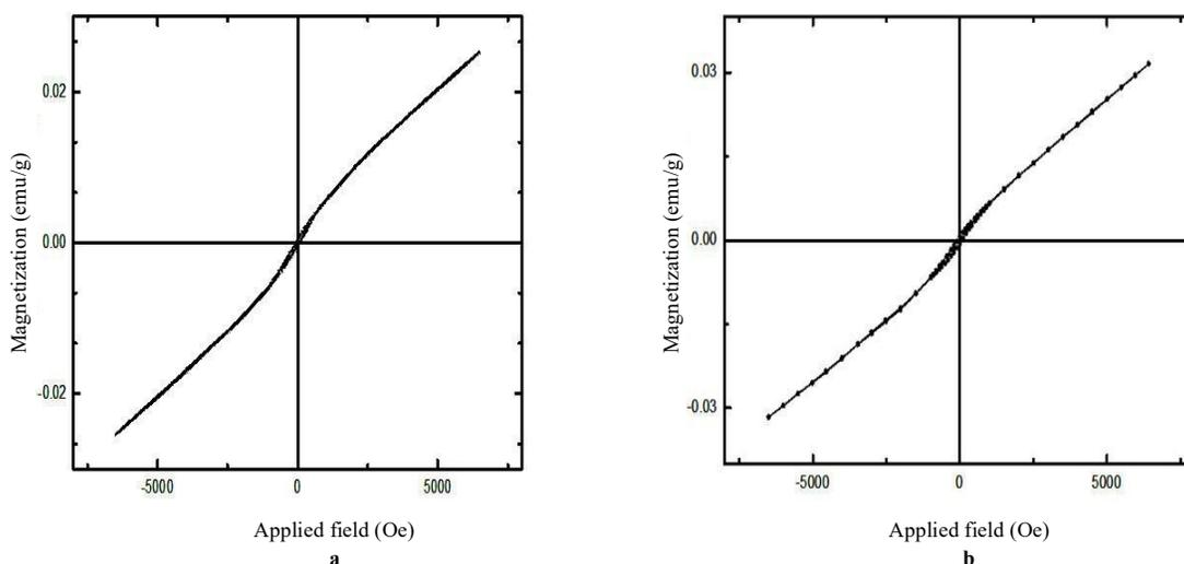
Fig. 6 magnetization of Fe-doped SnO<sub>2</sub> samples with (a) 4 wt% and (b) 7.93 wt% doping versus magnetic field
