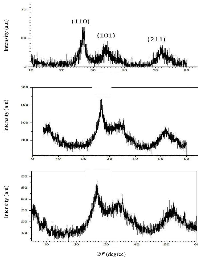
Fig. 1 XRD patterns of (a) undoped and Fe doped  $\text{SnO}_2$  samples with (b) 4% and (c) 7.93% doping
