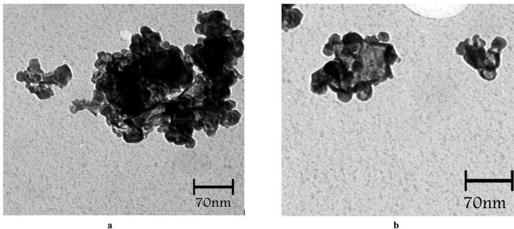
Fig. 5 TEM images (a) and (b) of SnO<sub>2</sub> nanoparticles (different regions)
