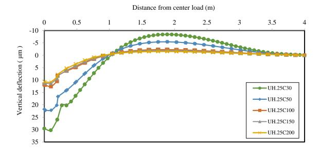
**Figure 8.** Vertical deflection of the pavement for various undrained shear strength of the subgrade when the reinforcement is placed at q=0.25 m.
