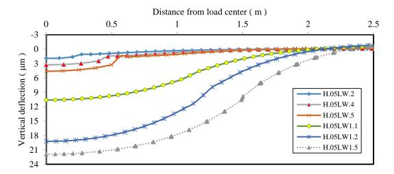
**Figure 4.** Vertical deflection of the pavement for various length of load area when the reinforcement is placed at q=0.05m.
