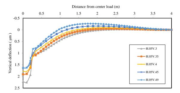
**Figure 10.** Variation of vertical surface deflection along horizontal direction for the models with various Poisson's ratios of the subgrade when the reinforcement is located at q=0.05 m.
