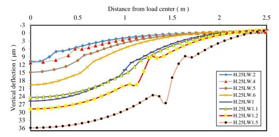
**Figure 5.** Vertical deflection of the pavement for various length of load area when the reinforcement is placed at q=0.25 m.
