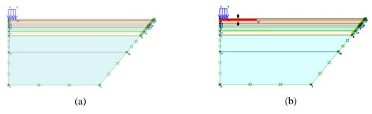
**Figure 2.** Geometry model and boundary conditions of the model; (a) without geogrid and (b) with geogrid reinforcement.
