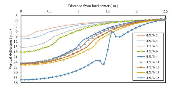
**Figure 6.** Vertical deflection of the pavement for various length of load area when the reinforcement is placed at q=0.5 m.
