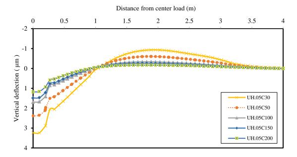
**Figure 7.** Vertical deflection of the pavement for various undrained shear strength of the subgrade when the reinforcement is placed at q=0.05 m.
