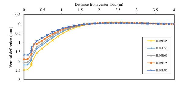
**Figure 11.** Variation of vertical surface deflection along horizontal direction for the models with various elasticity moduli of the subgrade when the reinforcement is located at q=0.05 m.
