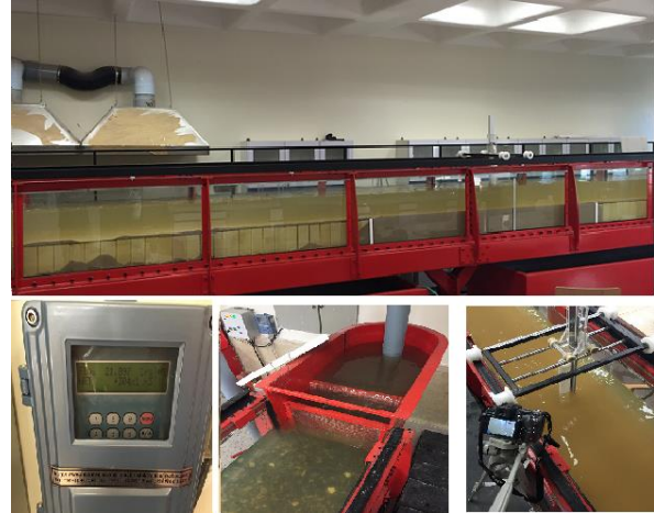
Fig. 2. The flume of hydraulics laboratory located on the Arak University; Below: (left) ultrasonic flow meter, (middle) stilling basin, (right) point gauge
