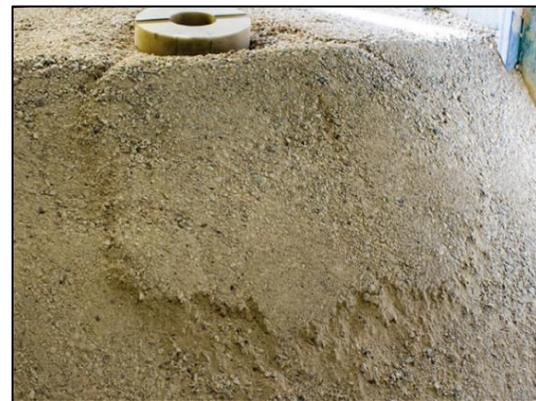
**Fig. 3.** Failure mode of ring footing
