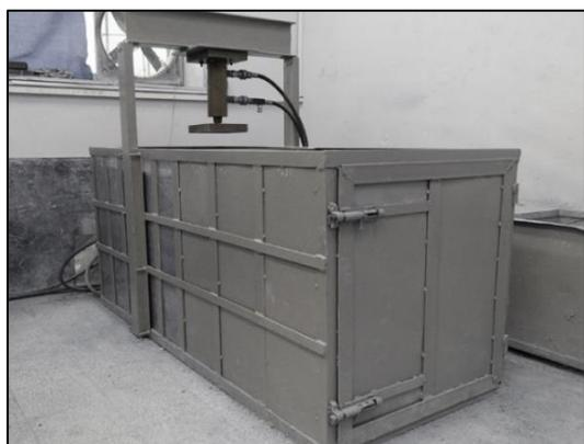
Fig. 2. Test box and loading apparatus.
