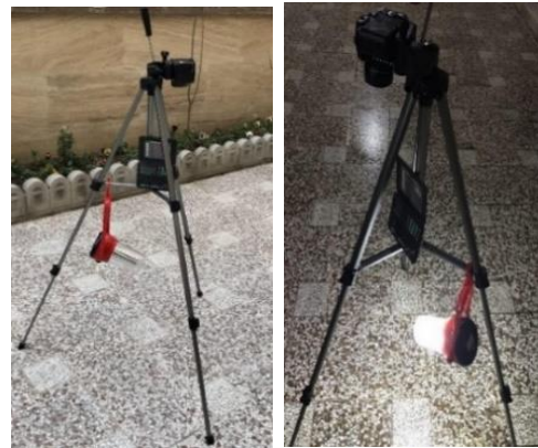
Fig. 7. The hardware used for pavement distress image capturing in controlled conditions.
