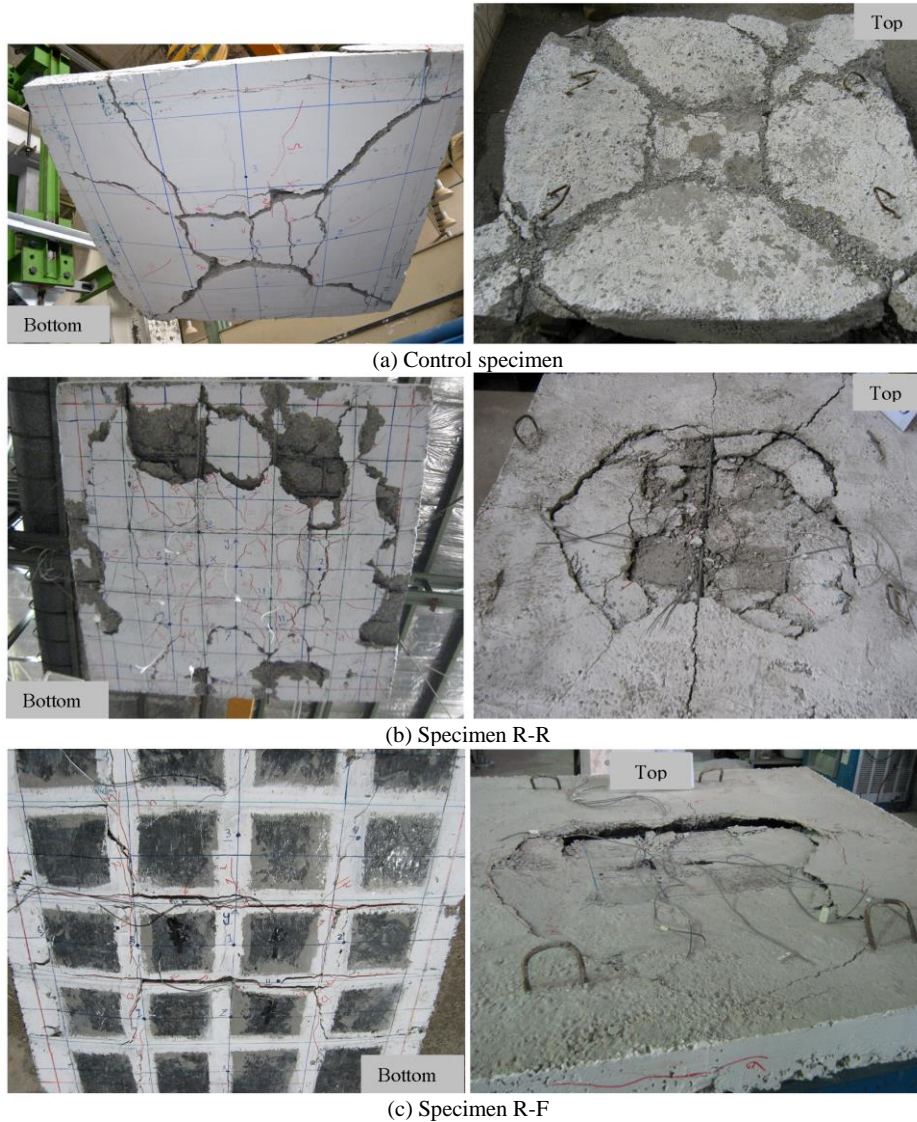
Figure 8. Cracking patterns of the specimens after failure.
