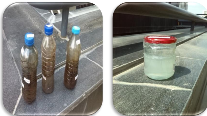
Fig. 17. Contaminated water samples accumulated from the surface of asphalt pavement.
