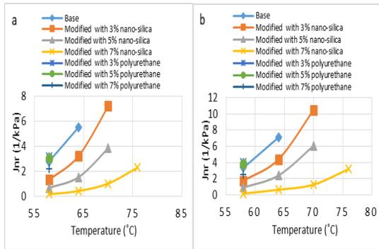
Fig. 2. Jnr Parameters at 0.1 kPa (a), 3.2 kPa (b).
