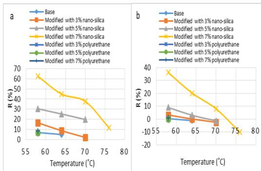
Fig. 3. Recovery parameters at 0.1 kPa (a), 3.2 kPa (b).
