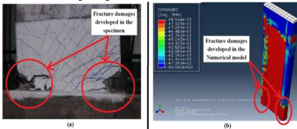
Fig. 3. Final failure appearance in the experimental specimen (a) and numerical model (b).
