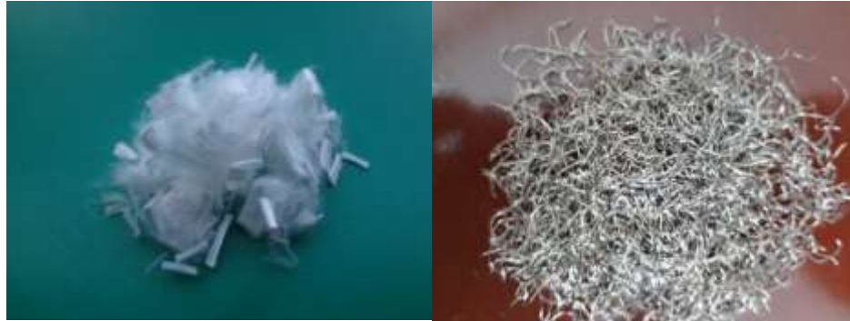
Fig. 1. Micro Steel and Polypropylene fibers.
