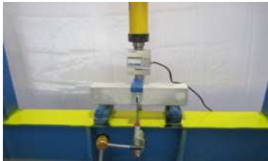
Fig. 6. Three point bending test setup.
