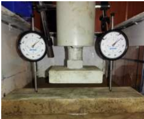
Fig. 3. Dial gauges in both sides of the footing.
