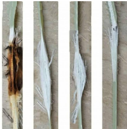
Fig. 4. Different failure modes of GFRP laminates at elevated temperatures
