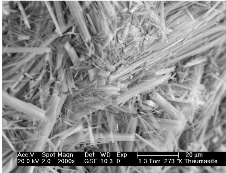
Fig. 3. SEM figures of the natural mineral thaumasite [41]
