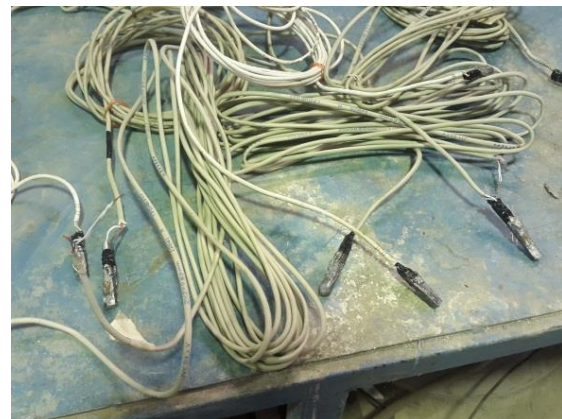
Fig. 6. Prepared strain gauge for installation on the planting rebar.
