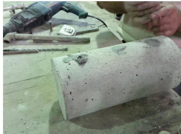
Fig. 2. Rebar planting process with glue
