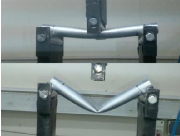
Fig. 6. Deformation of the inner tube during three-point bending test
