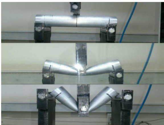
Fig. 7. Deformation of the outer tube during three-point bending test
