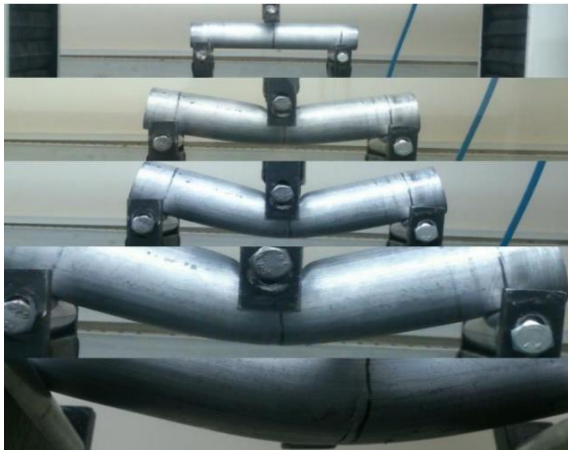
Fig. 8. Deformation of the FFD tube during three-point bending test (from start to fracture)
