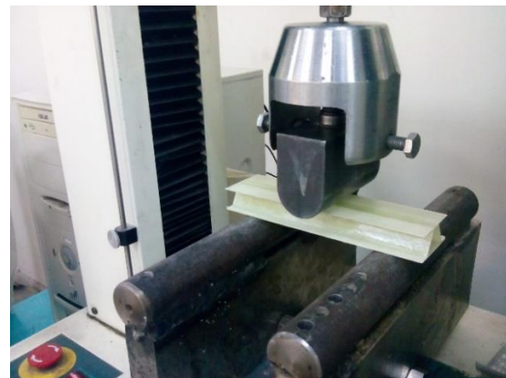
Fig. 14. HOUNSFIELD machine used for three-point bending test.
