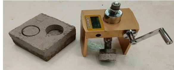
a) Determining the bond tensile strength
