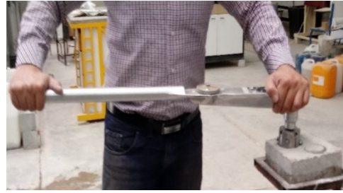
a) Determining the Bond shear strength
