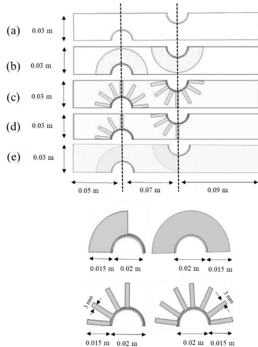
Figure 4. The geometrical dimensions of tubular-fin heat exchangers (a) without fin (b) circular fin (c) serrated fin (d) semi-serrated fin and (e) semi-circular fin.
