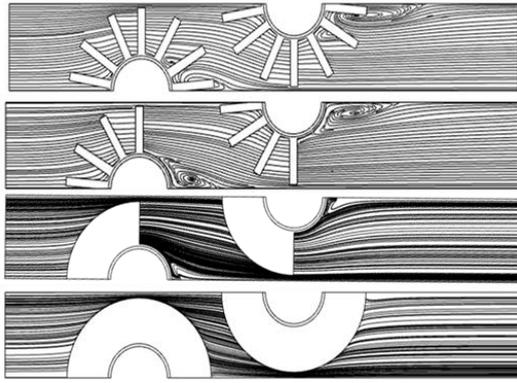
**Figure 15.** Streamlines for serrated, semi-serrated, semi-circular, and circular fins ( $Re = 28000$ ).
