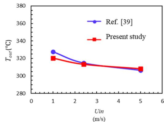
**Figure 5.** Comparison and validation of the results of the present study with reference [39] by calculating the outlet temperature for different inlet velocities.
