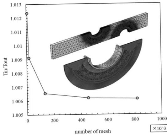
Figure 1. Sample of Mesh that used in the numerical modeling and mesh independence
