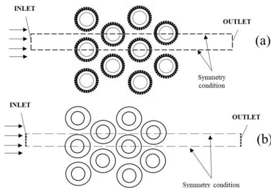
Figure 2. Side view of the studied tubular-fin heat exchanger with (a) serrated fins (b) circular fins
