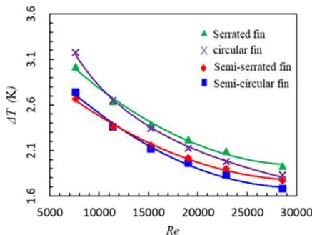
**Figure 8.** Inlet and outlet temperature difference with increasing Reynolds number for serrated, semi-serrated, circular and semi-circular fins.
