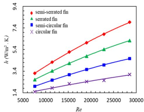
**Figure 9.** Variations of heat transfer coefficient (h) by the Reynolds number for serrated, semi-serrated, circular and semi-circular fins.
