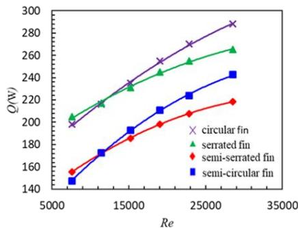
**Figure 7.** Heat transfer rate at different Reynolds numbers for serrated, semi-serrated, circular and semi-circular fins.
