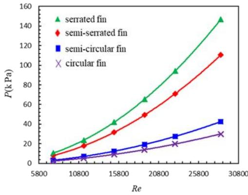
Figure 11. Pressure drop in different Reynolds for serrated, semi-serrated, circular, and semi-circular fins.
