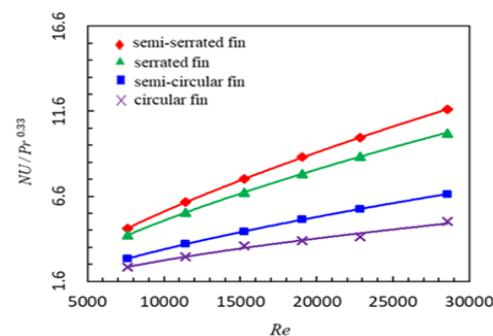
**Figure 10.** Nusselt number versus Reynolds number for serrated, semi-serrated circular, and semi-circular fins.
