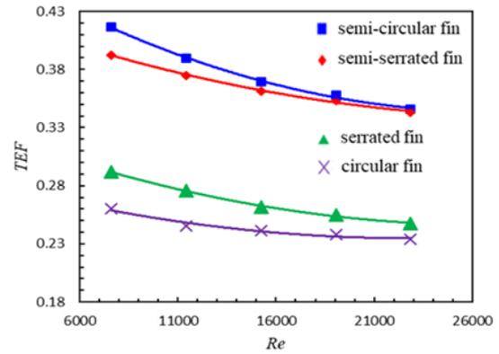
Figure12. TEF variations with Reynolds number for serrated, semi-serrated, circular, and semi-circular fins
