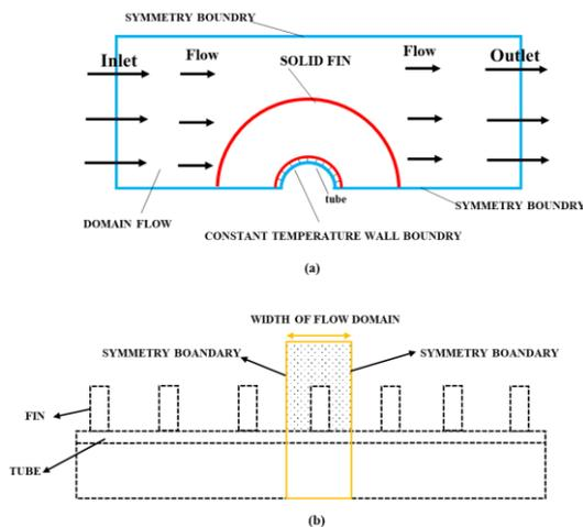
Figure 3. Boundary conditions for the studied geometry from (a) side view and (b) front view.
