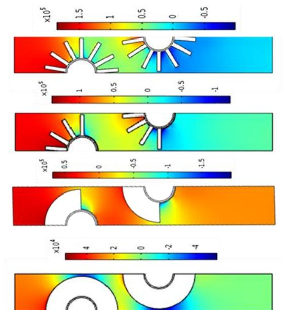
Figure14: Pressure contour [Pa] in Reynolds almost 28000 for serrated, semi-serrated, semi-circular and circular fins.
