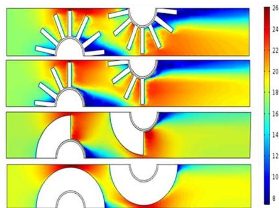
Figure13. Contour of gas velocity [m/s] in Reynolds almost 28000 for serrated, semi-serrated, semi-circular, and circular fins.
