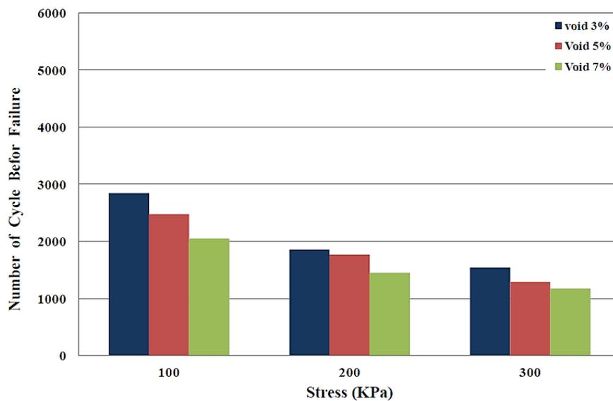
**Fig.2.** Failure cycle number versus stress for 85/100 bitumen-built silica-material samples with air void contents of 3%, 5%, and 7%.
