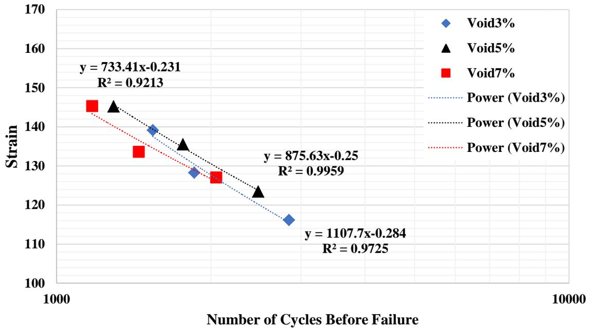
Fig.3. Failure cycle number versus ultimate strain for 85/100 bitumen-built silica-material asphalt samples.
