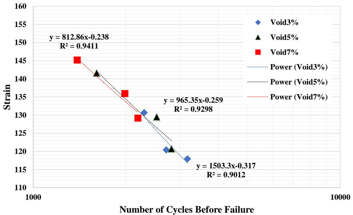
Fig. 8. Failure cycle number versus ultimate strain for 85/100 bitumen-built lime-material asphalt samples.
