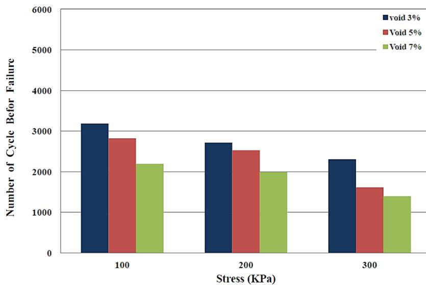
**Fig. 6.** Failure cycle number versus stress for 85/100 bitumen-built lime-material samples with air void contents of 3%, 5%, and 7%.
