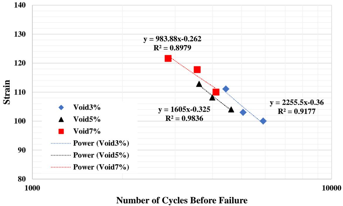
Fig. 7. Failure cycle number versus ultimate strain for 60/70 bitumen-built lime-material asphalt samples.
