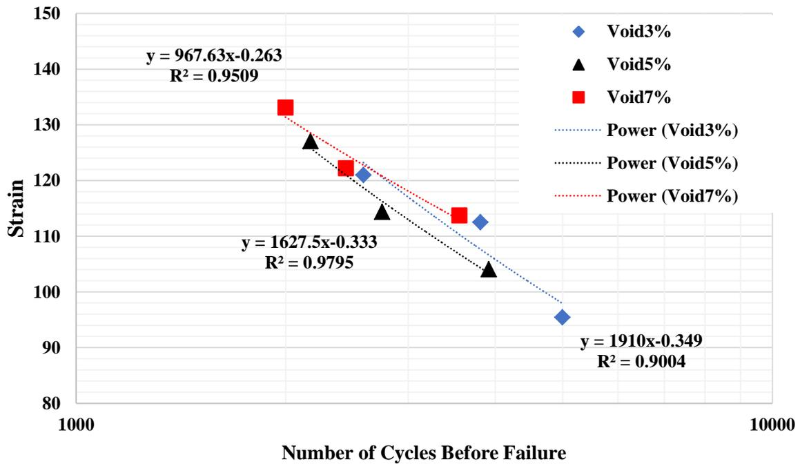
Fig.4. Failure cycle number versus ultimate strain for 60/70 bitumen-built silica-material asphalt samples.
