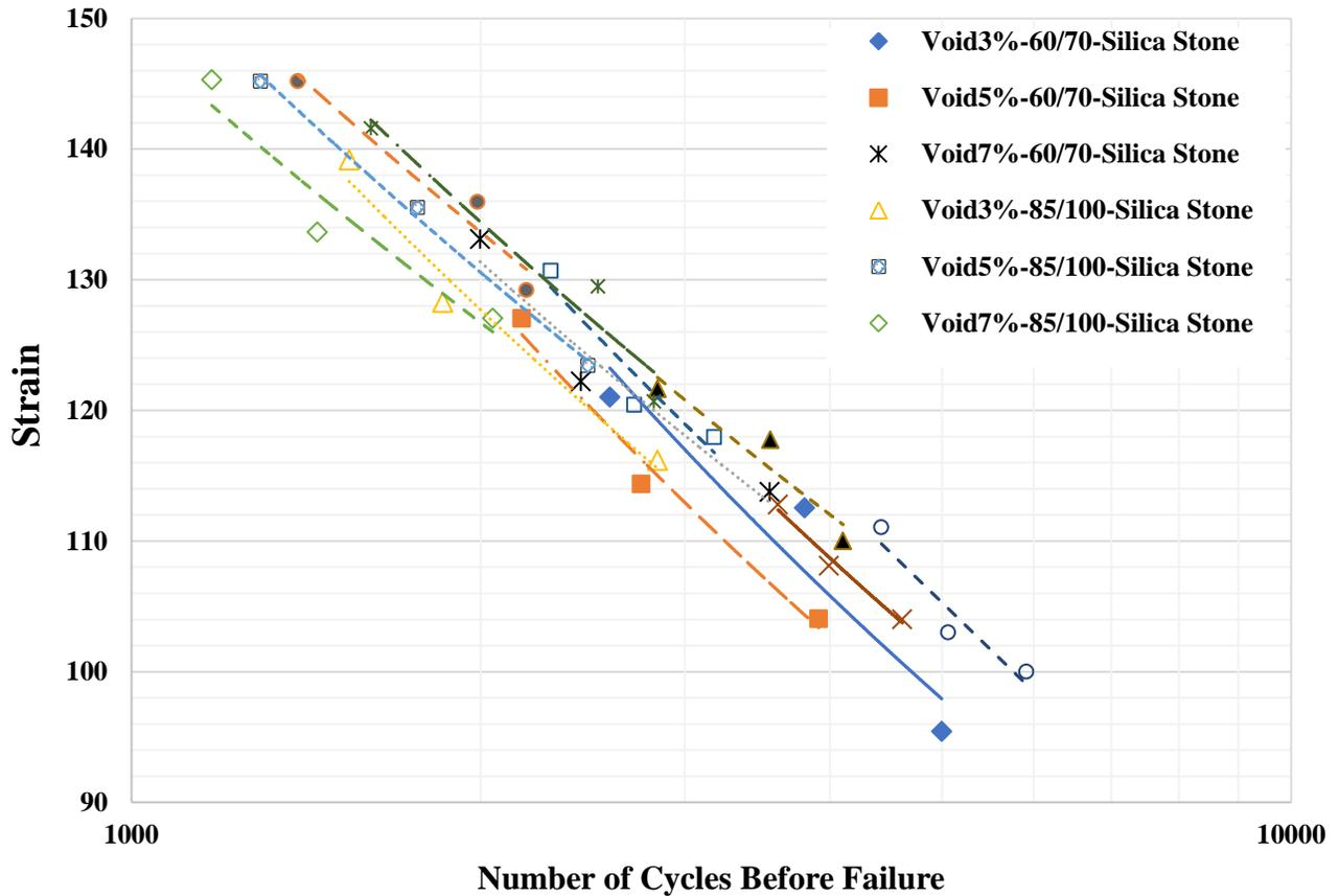
Fig. 9. Failure cycle number versus ultimate strain for asphalt samples of this study.
