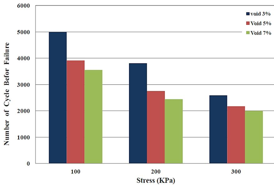
**Fig. 1.** Failure cycle number versus stress for 60/70 bitumen-built silica-material samples with air void contents of 3%, 5%, and 7%.
