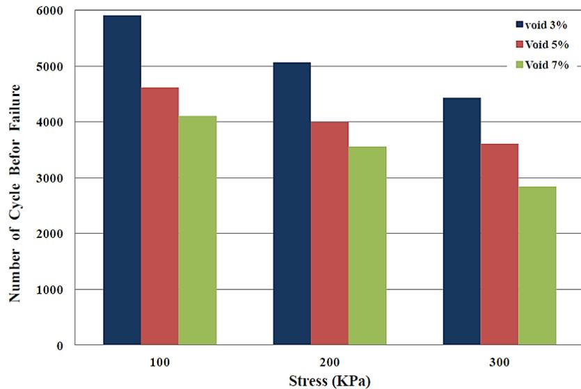
**Fig. 5.** Failure cycle number versus stress for 60/70 bitumen-built lime-material samples with air void contents of 3%, 5%, and 7%.
