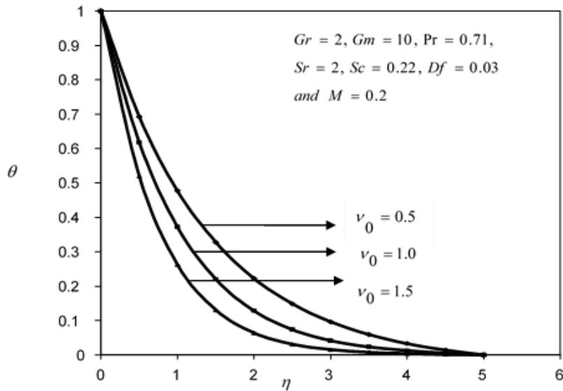
Fig. 5. Temperature profiles for different values of  $v_0$
