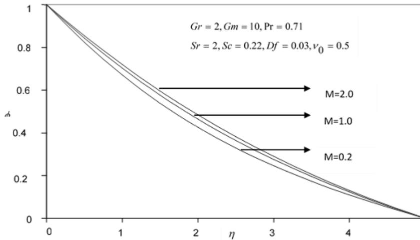
Fig. 11. Concentration profiles for different values of M.
