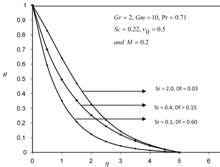
Fig. 6. Temperature profiles for different values of  $Sr$
