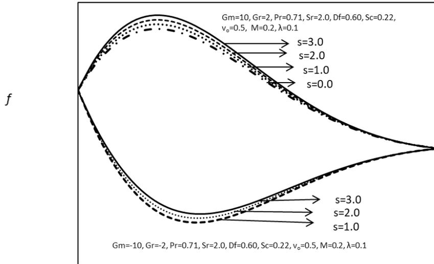
Fig. 4. Velocity profiles for different values of  $s$ .
