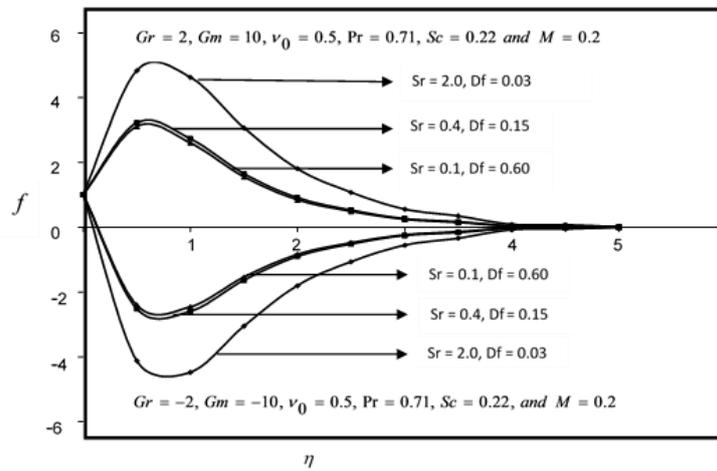
Fig. 2. Velocity profiles for different values of  $Sr$  and  $Df$ .
