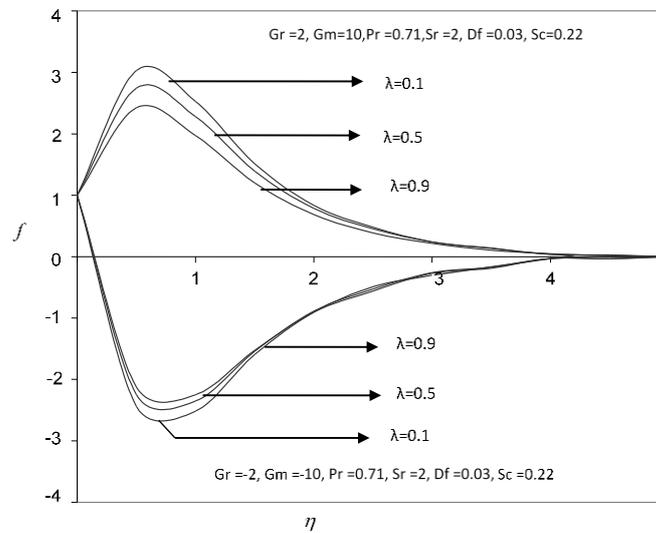
Fig. 3. Velocity profiles for different values of  $\lambda$ .
