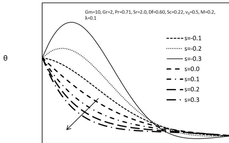
Fig. 8. Temperature profiles for positive and negative values of s.
