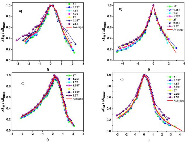
Fig. 1. Universal behavior of the scaled entropy change curves of the samples x=0 (a), x=0.0125 (b), x=0.05 (c) and x=0.1 (d)
