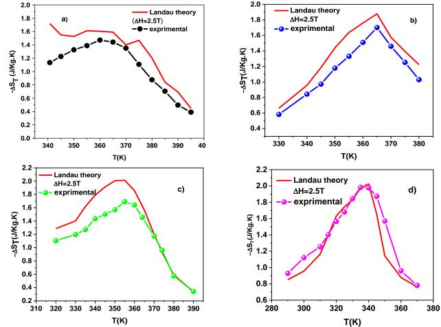
**Fig. 3**. Temperature dependence of the magnetic entropy change derived from magnetic measurements estimated by the Landau theory at the applied magnetic fields for samples x=0 (a), x=0.0125 (b), x=0.05 (c) and x=0.1 (d)
