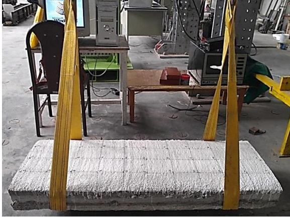
Fig. 5. Hanged position of the prestressed concrete slab specimen for performing modal testing [56].
